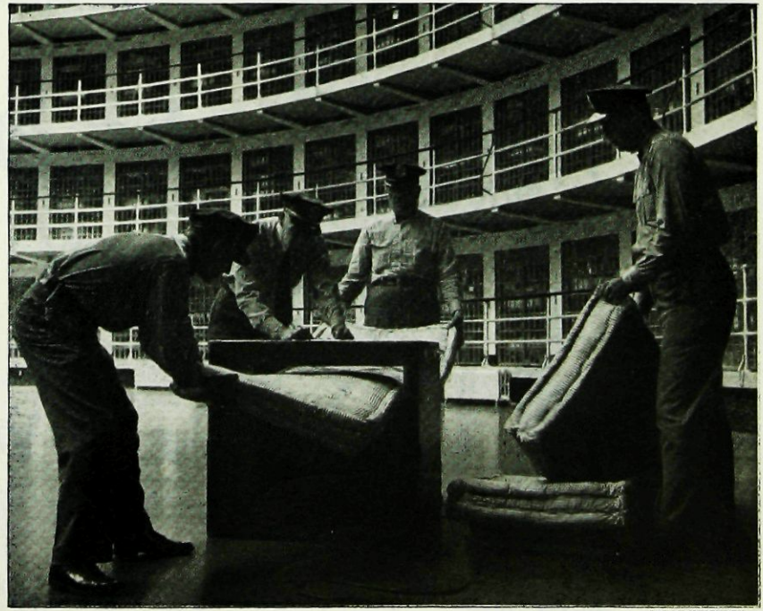
During a surprise cell shakedown, guards run prisoners' mattresses through a machine that detects any metallic objects which might be concealed in the stuffing.
