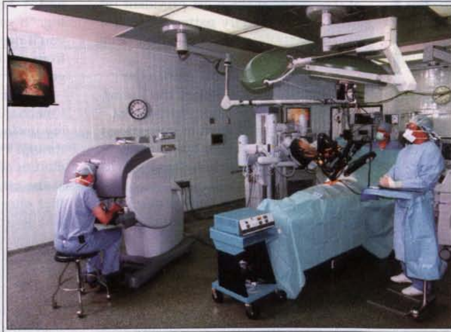
Surgeons manipulate robotic hands via remote control to perform a da Vinci prostatectomy. The new surgical technique is designed to reduce blood loss, scarring, and pain, and promote faster recovery. Patients are typically discharged within 24 hours.
