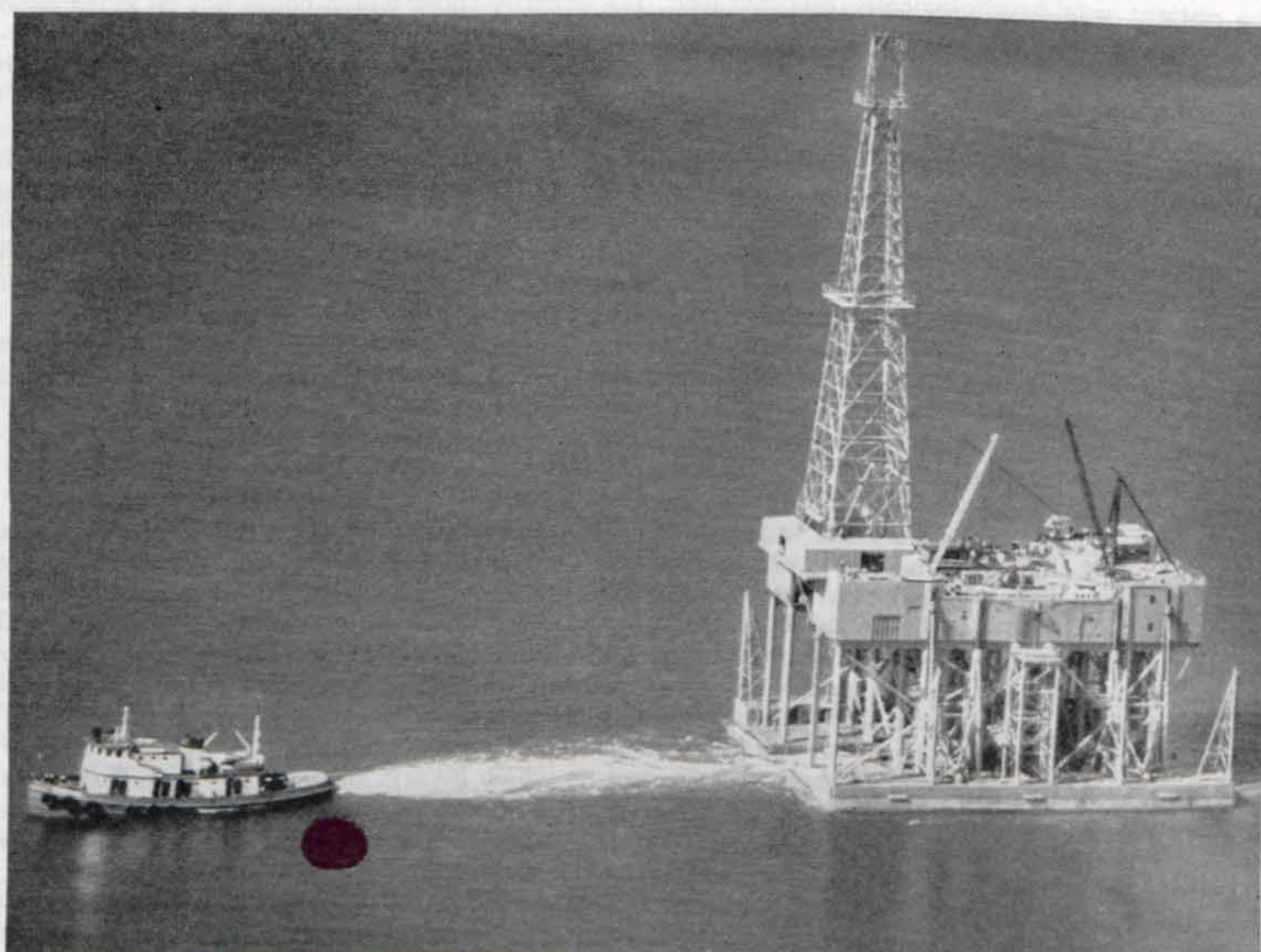
Kermac 44, a submersible barge. When this monster is operating—at a cost of thousands of dollars a day—its hull sits on the gulf floor. Its drill can reach a depth of three miles. INGALLS SHIPBUILDING CORP.
